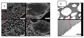
Figure 1: porous nanocomposite films a) at the SEM scale and b) at the TEM scale on an ultra-microtomed slice.
